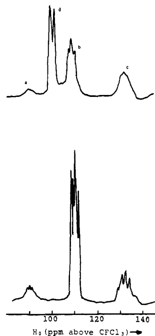
Figure 1. Fluorine (56.4 MHz) spectrum of ethyl fluoride-5.0 \text{SbF}_5 \cdot \text{SO}_2 at -85^\circ (top). Fluorine spectrum of ethyl fluoride-1.3 \text{SbF}_5 \cdot \text{SO}_2 at -90^\circ (bottom).
